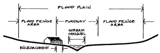
Figure 12.2, Flood Plain Cross-Section
