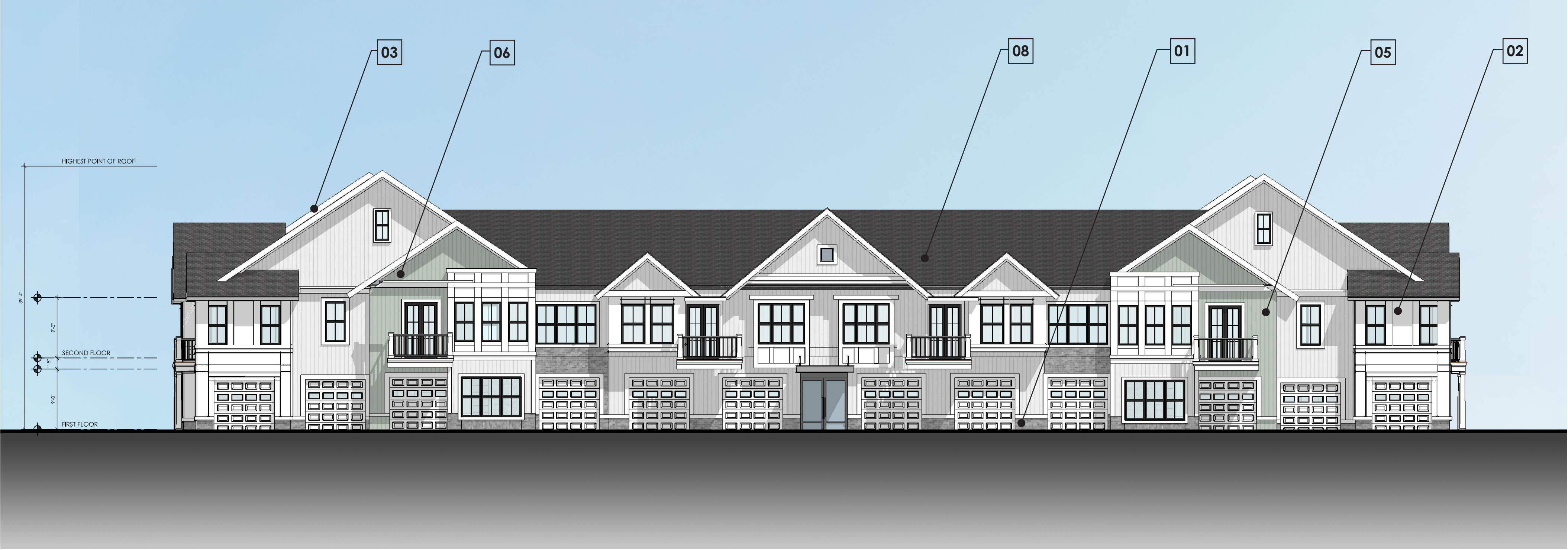
01 SOUTH BUILDING ELEVATION SCALE: 1/16" = 1'-0" 16'-0" 32'-0" 48'-0"
