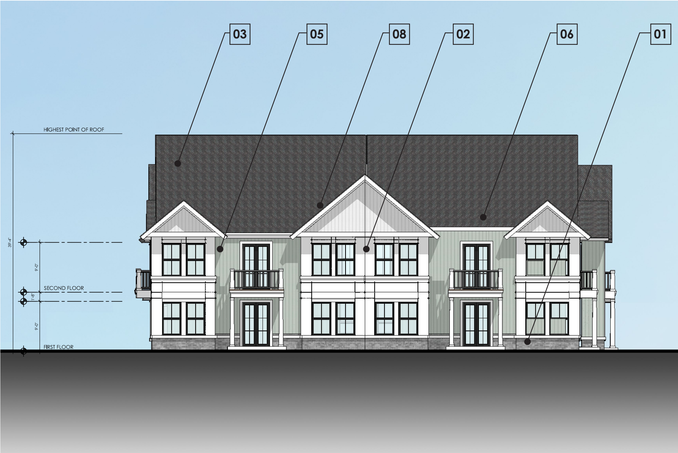
02 EAST BUILDING ELEVATION SCALE: 3/32" = 1'-0"
