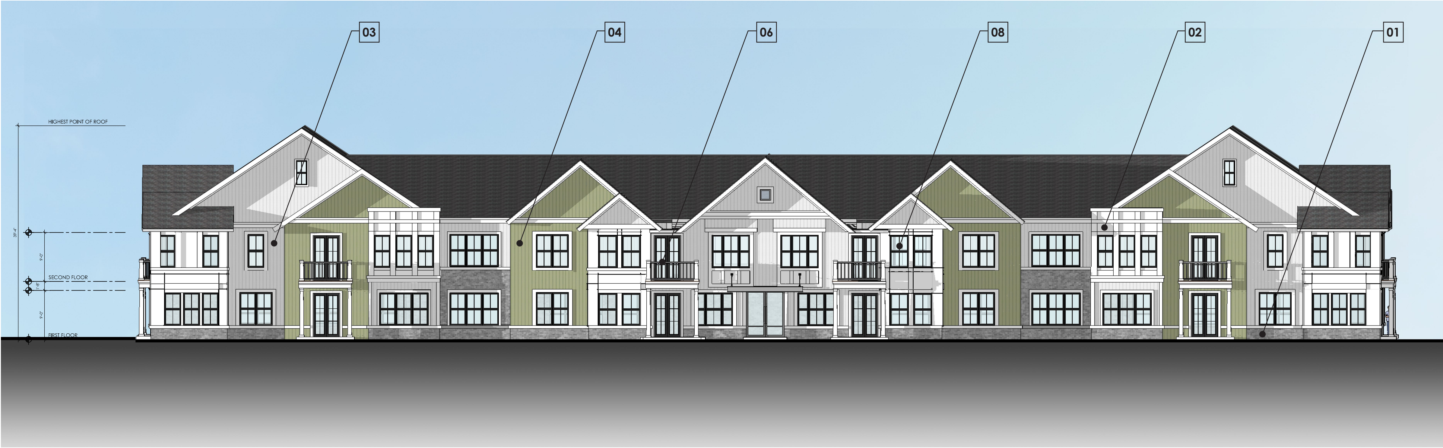
01 NORTH BUILDING ELEVATION SCALE: 1/16" = 1'-0" 16'-0" 32'-0" 48'-0"
