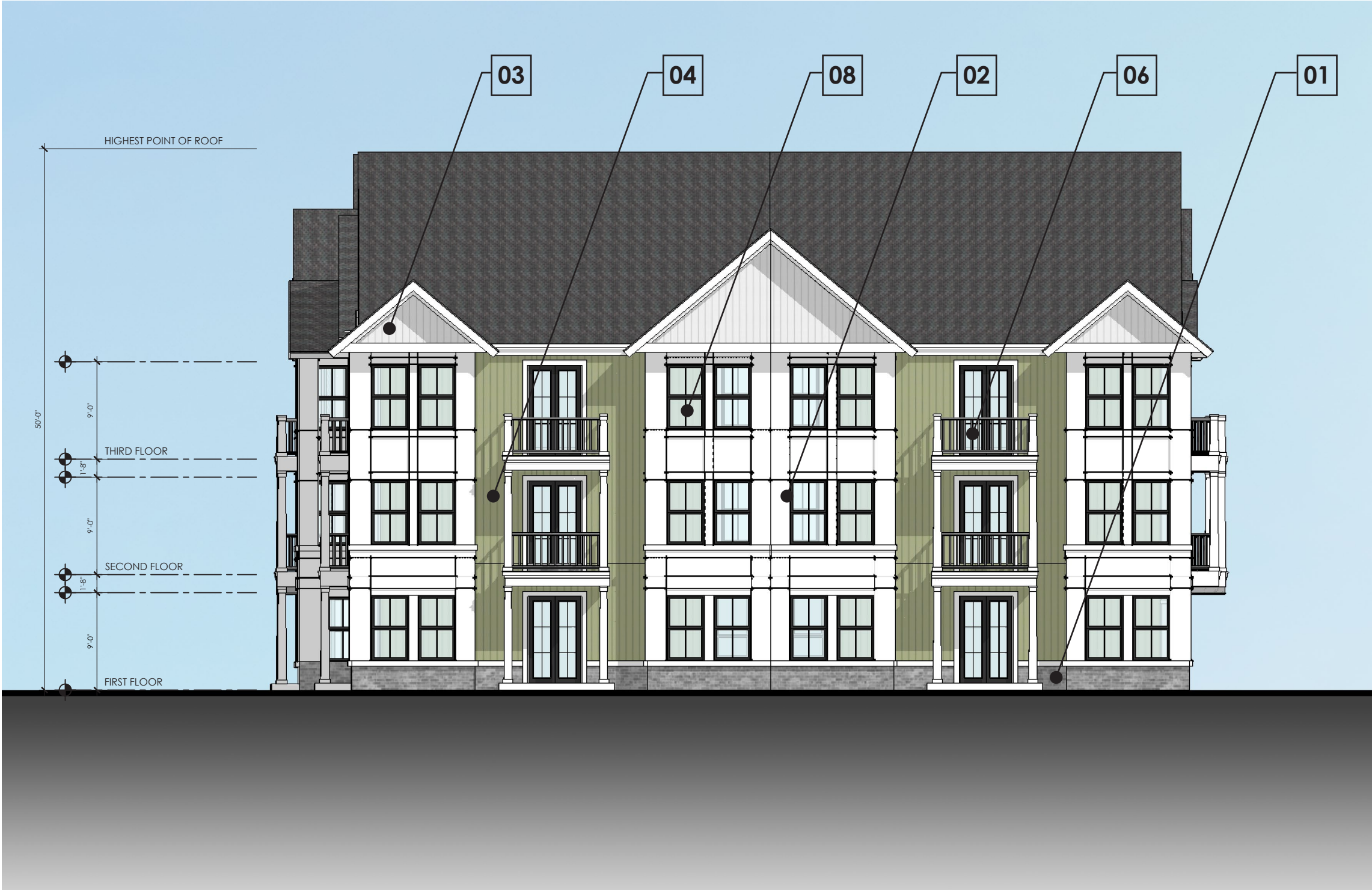
02 WEST BUILDING ELEVATION SCALE: 3/32" = 1'-0"
